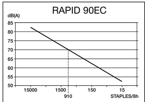
Equivalent noise level dB(A) at maximum capacity and power.
